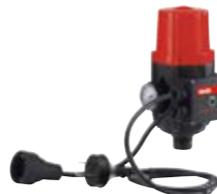
The Hydrocontrol automatically converts your existing transfer pump into a household water supply pump. It is easily fitted to any Jet pump with a 1" thread and will switch the pump on and off as you turn your tap on and off. Additionally, the Hydrocontrol will check pressure lines for leaks and has dry run protection should the water supply run out.
